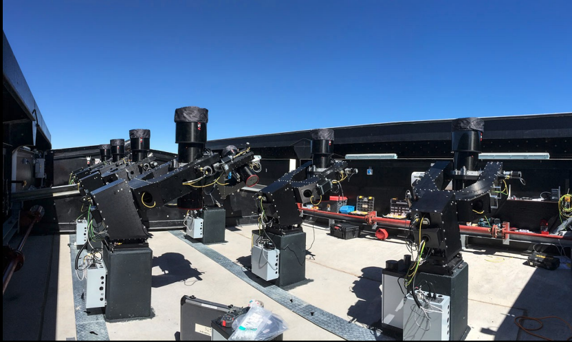
Next Generation Transit Survey (NGTS): 20 cm'lik 12 teleskop → 96 \square^\circ , 5"/piksel, Şili Paranal 2016 - ?, 25 gezegen!
